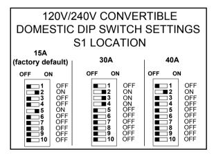
\*\*Dip switch #9 must be OFF for a 1-pump model
