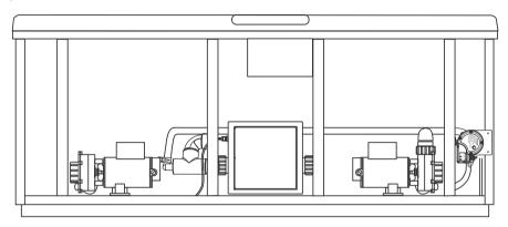
**Figure 12:** Spa equipment compartment (Spa features subject to change without notice. Component locations vary by model.)
