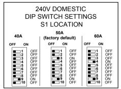
Dip switch #9 must be ON for a 2-pump model
