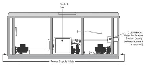
**Figure 15:** Spa equipment compartment (Spa features subject to change without notice. Component locations vary by model.)
