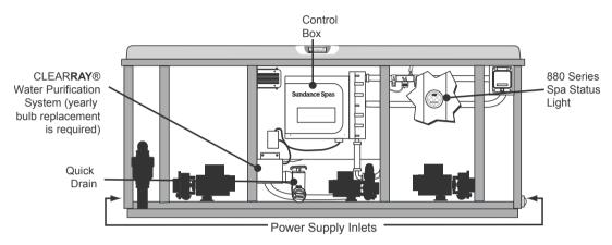
**Figure 6:** Spa equipment compartment (Spa features subject to change without notice. Component locations vary by model.)
