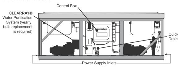
**Figure 3:** Spa equipment compartment (Spa features subject to change without notice. Component locations vary by model.)
